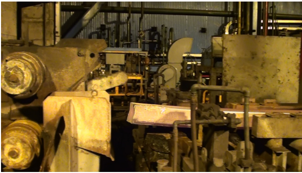
Fig.4. Bloom entered second stage rolling station.
